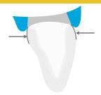
A digital scan should capture the entire restorative margin as well as about 0.5mm of the tooth/root surface apical to the margin for fabrication of the correct emergence profile. This profile needs to be smooth to create a restoration/tooth junction that is biologically sound and not prone to plaque accumulation. Effective retraction will facilitate this (see below).
